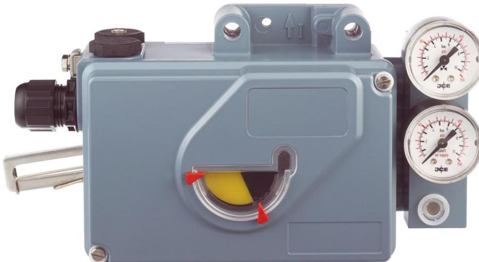
Analog positioner type SRI990 with analog input 4 - 20mA is designed to control pneumatic valves. The main advantage is simple settings using switches and potentiometers. Modular structure allows the simple reconstruction to intelligent device based on the exchange of electronics.
